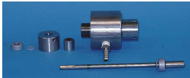
5. Pull the drive shaft out of the unit.
