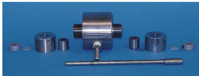
6. Remove right side threaded end cap (may need pliers) by rotating counterclockwise.
