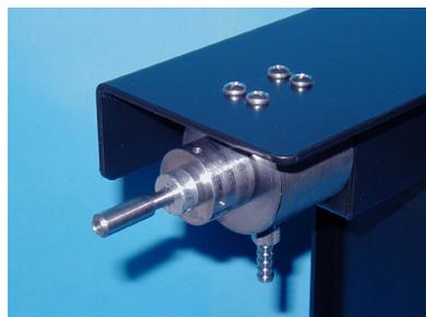
1. Unplug the Kugelrohr vacuum drive unit and place into a fume hood.
