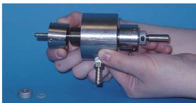
4. Remove left side threaded end cap (may need pliers) by rotating counterclockwise.
